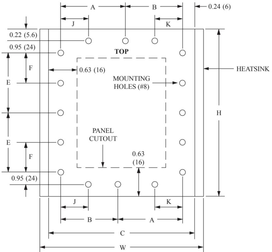
**THROUGH-HOLE MOUNT DIMENSIONS FOR MODELS UP TO 10 HP (7.5 kW)**
