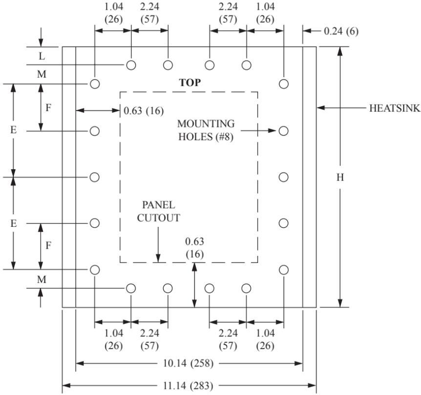
**THROUGH-HOLE CUTOUT DIMENSIONS FOR 15 HP (11 kW) & 20 HP (15 kW) MODELS**
