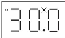
Pressing the **Mode** will store the new setting and also exit the PROGRAM mode. To change another parameter, press the **Mode** key again to re-enter the PROGRAM mode (the parameter menu will be accessed at the parameter that was last viewed or changed before exiting). If the **Mode** key is pressed within two minutes of exiting the PROGRAM mode, the password is not required access the parameters. After two minutes, the password must be entered in order to access the parameters again.
